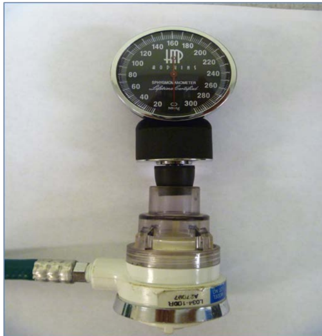
Figure 1. Demand valve test kit assembled for testing
